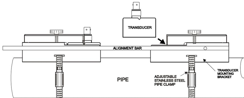
Mount the Mounting Bracket as illustrated on pipes 2" / 50 mm OD or larger. Stainless steel bands are included for mounting on pipes up to 30" / 750 mm OD.
