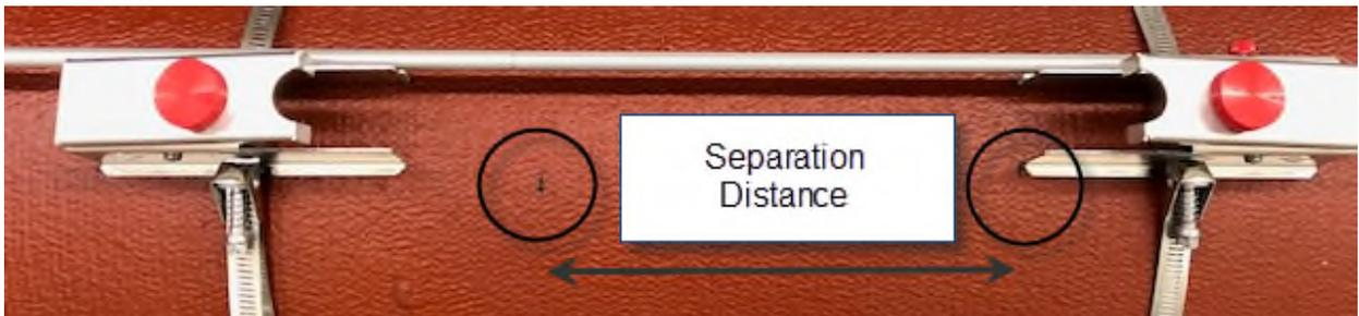
6. Move the non-permanent bracket to position at the mark you created at step 5, and tighten it completely. Apply coupling compound to the transducers, and install them in the brackets.
