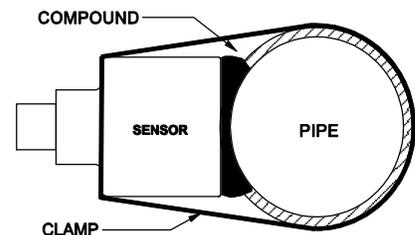
Over time temporary coupling compounds (e.g. Petroleum Gel) may gradually sag away from the sensor resulting in reduced signal strength and finally complete loss of signal. Warm temperatures, moisture and vibration will accelerate this process. Super Lube® as supplied with the TTFM 6.1 (and available from Greyline Instruments or home improvement stores) is recommended for permanent installations.
