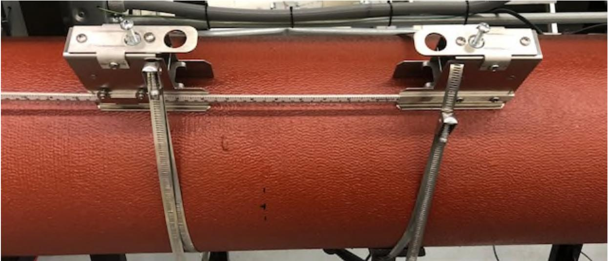
5. Apply coupling compound to the transducers, and install them in the brackets.
