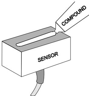
Use the pipe clamp and rail (supplied) as illustrated on previous page. Apply Super Lube® to the colored face of the sensor. A bead, similar to toothpaste on a toothbrush, is ideal. Do not overtighten (crush the sensor).
