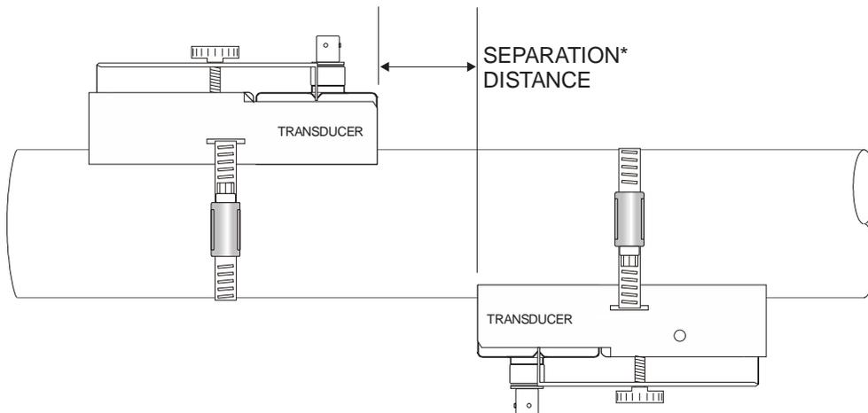
\* Shown in 'Setup' menu after sensor, fluid and pipe parameters are entered.
