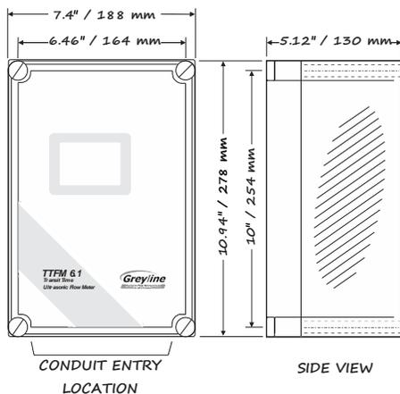
Note: This non-metallic enclosure does not automatically provide grounding between conduit connections. Grounding must be provided as part of the installation. Ground in accordance with the requirements of the National Electrical Code. System grounding is provided by connecting grounding wires from all conduit entries to the steel mounting plate or another point which provides continuity.
