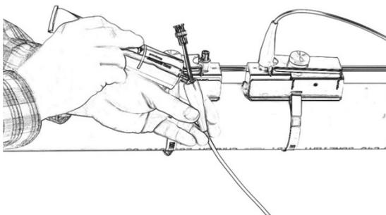
The TTFM 6.1 Transit Time Flowmeter transducers are rated for accidental submersion up to 10 psi (0.75 bar). The flowmeter will continue to operate and measure flow accurately during periods of submergence. Plastic seal jackets on the cables must be filled with coupling compound to provide additional moisture protection for the BNC cable connectors.
