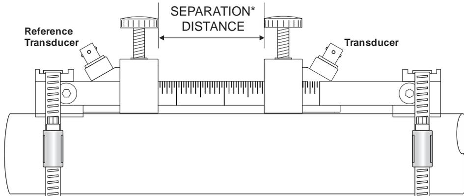
\* Shown in 'Setup' menu after sensor, fluid and pipe parameters are entered.
