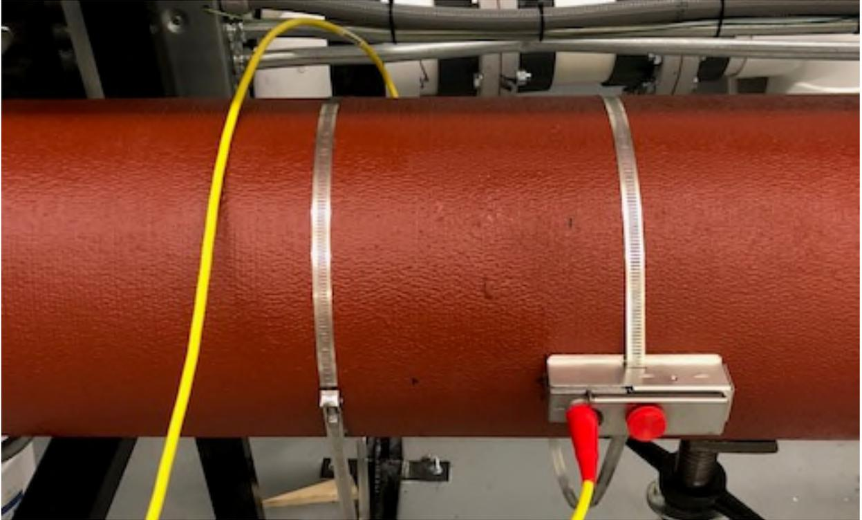
10. If you need to make fine adjustments ( $\pm 0.25''$ ) to the spacing at this point, you may do so by loosening the hose clamps slightly, and sliding the brackets while the transducers are installed inside them. Tighten the hose clamps when done.
