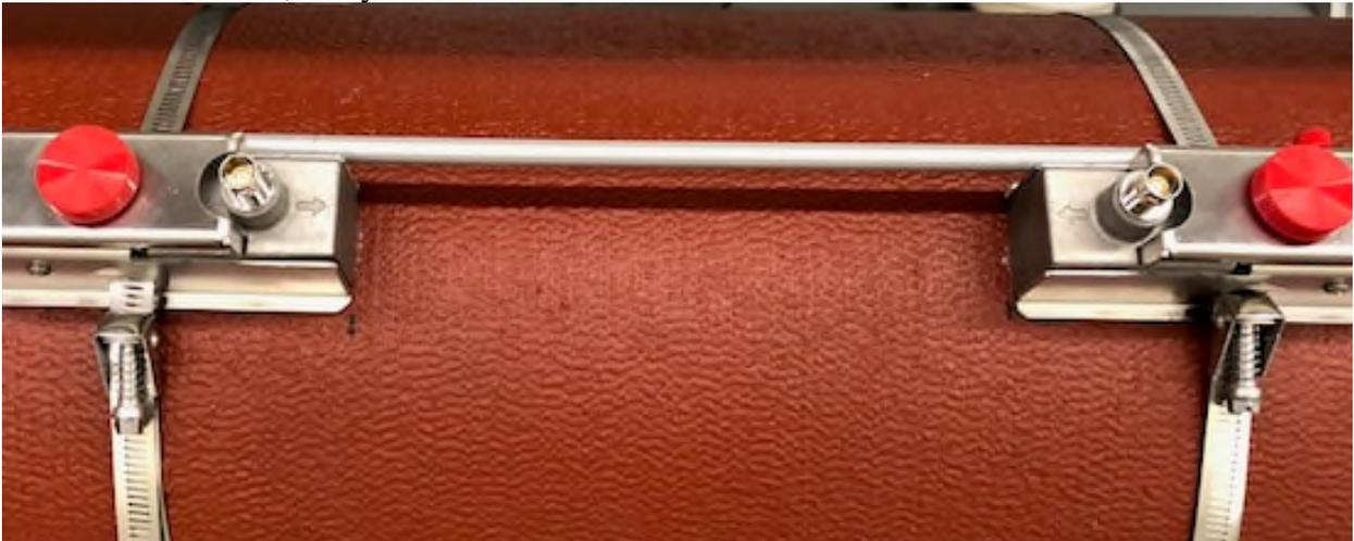
7. If you need to make fine adjustments ( $\pm 0.25''$ ) to the spacing at this point, you may do so by loosening the hose clamps slightly, and sliding the brackets while the transducers are installed inside them. Tighten hose clamps when done.
