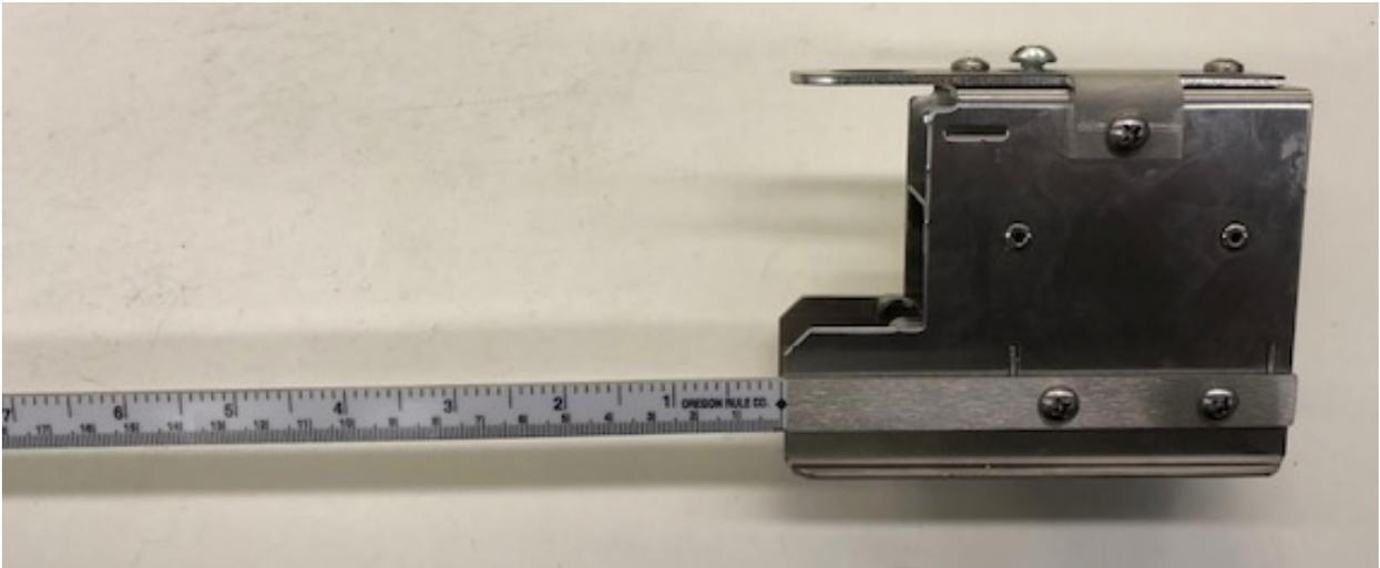
3. Insert the spacer bar into the left bracket, and position the bracket at the separation distance referenced earlier. Tighten the spacer bar clamp at this position:
