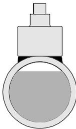
Avoid debris traveling at the bottom of a horizontal pipe.
